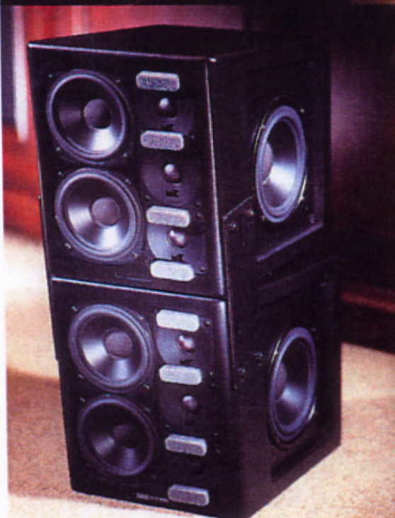
To meet the required SPL of 115dB, two M&K MPS-2550 Pro subwoofers were braced together for each of the left, center, and right channels. This unusual configuration resulted in a total system output increase of 6dB per channel.
